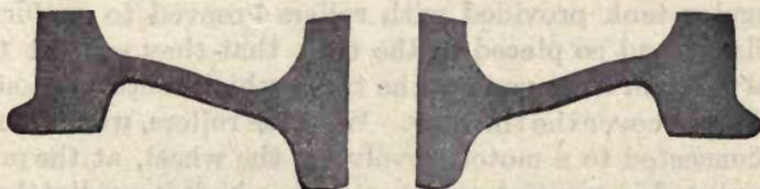
D. Wheel, after Punching, Rolling and Coning.
