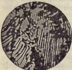
4. Laminated Pearlite. Cementite is completely segregated. Obtained by slow cooling.
