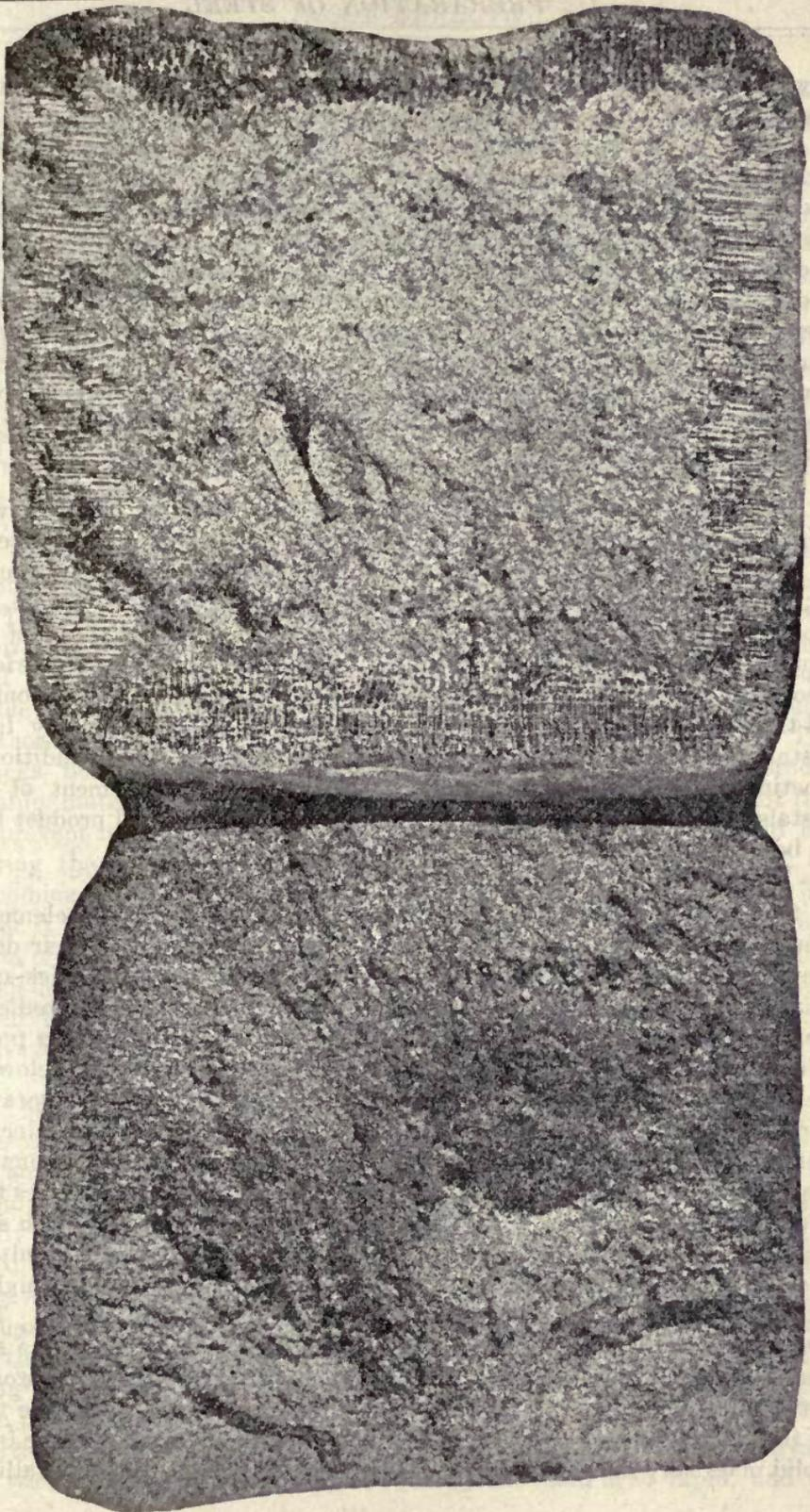
FIG. 56. Transverse Sections of Ingots Showing Blow Holes
